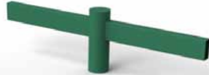
PROYECT 2 Straight rectangular-section double arm measuring 1.20 m in length for 2 or 3 floodlights. Fitting for columns with a tip diameter of 78 mm.
